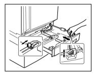
For "12-1/4 x 18" paper, adjust the trailing-edge guides as shown in the illustration.
